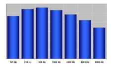
Figure 2: Average octave band spectrum of a male speaker
