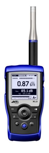
The XL2 Analyzer measures the speech intelligibility according to the latest revision of standard IEC 60268-16:2011 (edition 4) and older editions. It includes ambient noise correction and automated averaging of measurements. The XL2 displays the measurement results as STI or as CIS results, accompanied by the individual levels and modulation indices of the seven octave bands.
